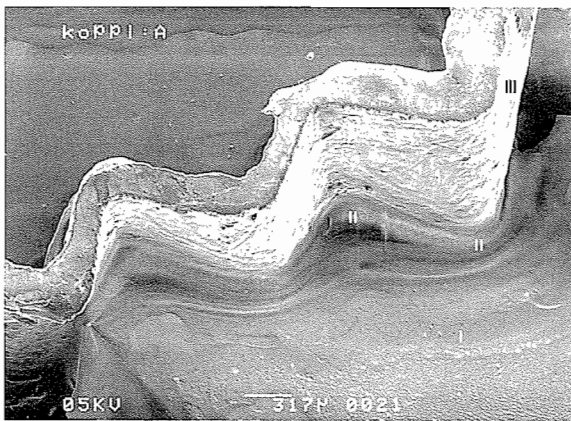
Figure 2. SEM photograph of head-plate A. Magnification 31.5 ×. I = gold sheet, II = soldering seam, and III = cell wall (photo GIA).
